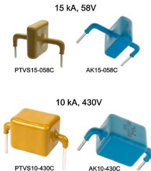
Fig. 7. High-power bidirectional transient voltage suppressors 58V, 15 kA (for input circuits protection – coils direction) and 430V 10 kA (for output circuits protection – reed switches or thyristors direction) manufactured by Bourns (left) and Littelfuse (right) companies.
